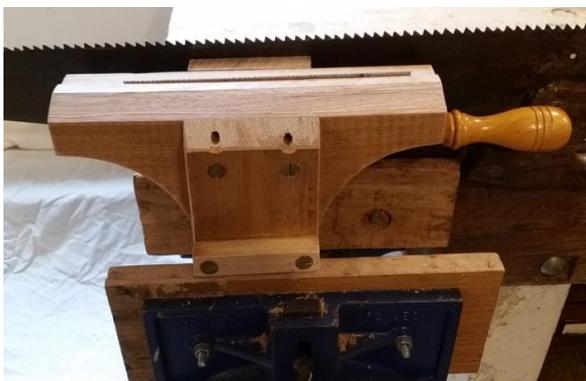
The photo on the left shows a dovetail saw mounted in the jaws, with the rip saw from the previous photo in the background to show the scale. The wood in this vice is in its third life. It was originally shelving in a chemist shop, it was
