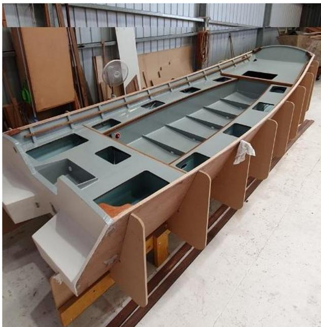
Interior view on the left and below the boat upside down with 3 coats of 2 pack epoxy primer completed.
