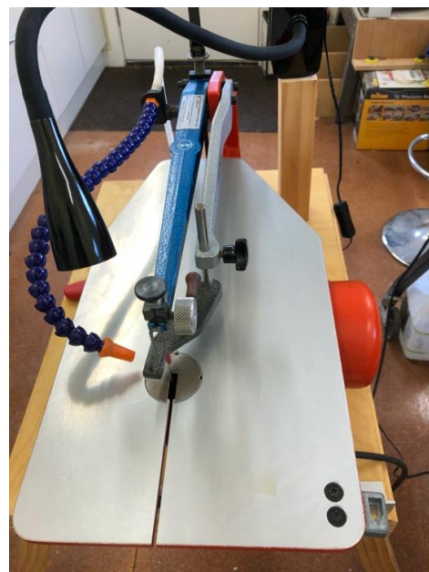
The quick release clamp is the silver coloured knob and the hold down is the dark grey arm near the blade.
