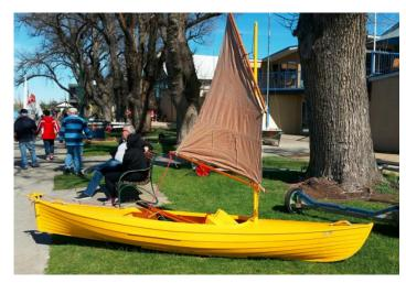
One person sea kayak, 5.2m long by 0.6m wide. Fast and stable with fore and aft hatches. Stitch and glue construction with hoop pine for the bottom and sides and gaboon ply for the deck and a lifting rudder with foot controls.
